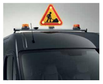
TriFlash triangles and SESALY flashing lights are designed for emergency response vehicles, works vehicles and service vehicles on public highways which are required to have suitable, regulatory signage. The triangle is made of light aluminium and polyamide with new generation 3D LED lights for optimum visibility and service life. Easy to install using a special adhesive.
