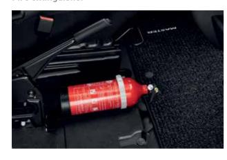
2 kg fire extinguisher with pressure gauge
