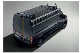
The ErgoRack rotating ladder carrier enables you to carry and handle any type of ladder effortlessly. Easy to install thanks to its compatibility with Renault roof bars, this system is made of light aluminium and is specially designed to avoid back injuries when loading and unloading through the use of its assisted system, reducing human effort required by half. Nude chassis incompatible.
