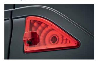
View the area behind your vehicle with reverse gear engaged.
